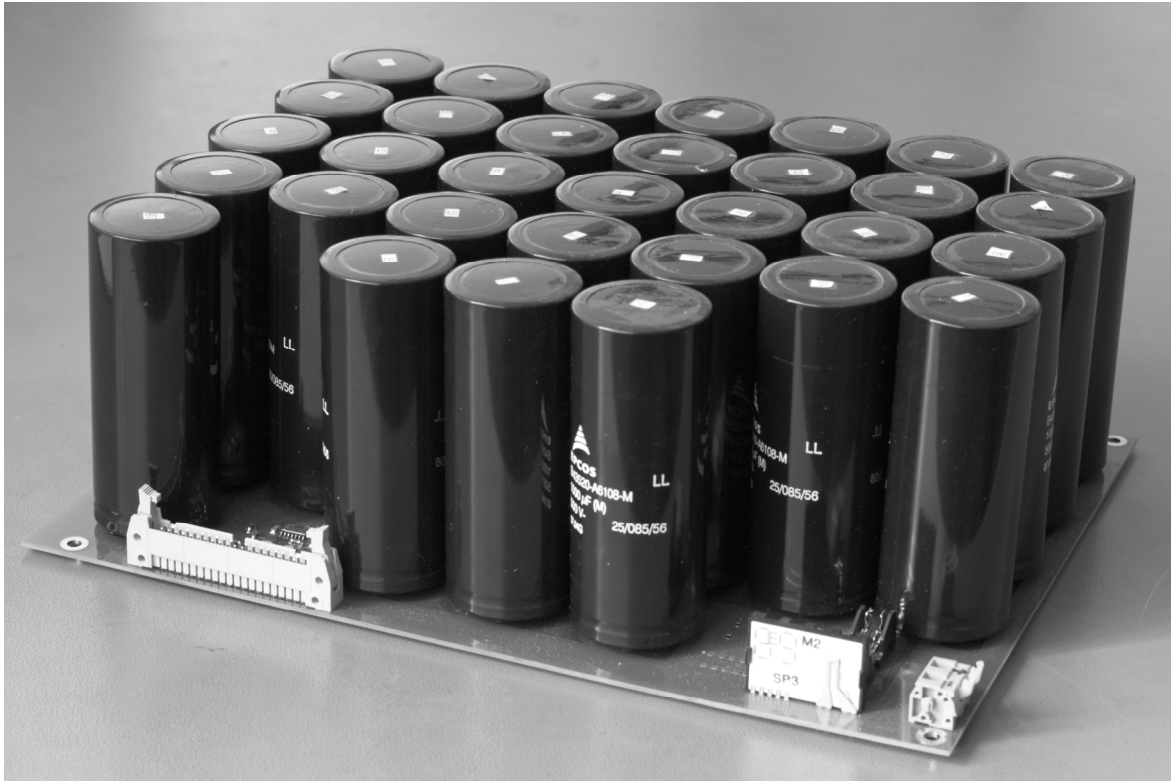
Figure 61: DC-Link of the prototype unit
