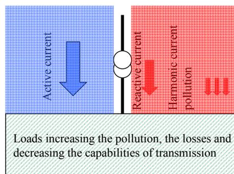
**Figure 2 Line pollution due to non-linear loads**
