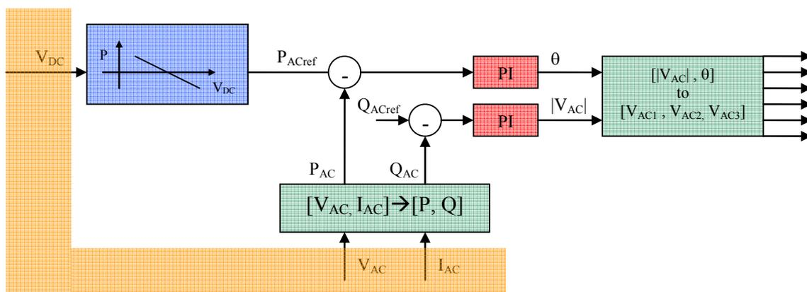
Figure 12: Voltage of the  $\mu$ Grid control
