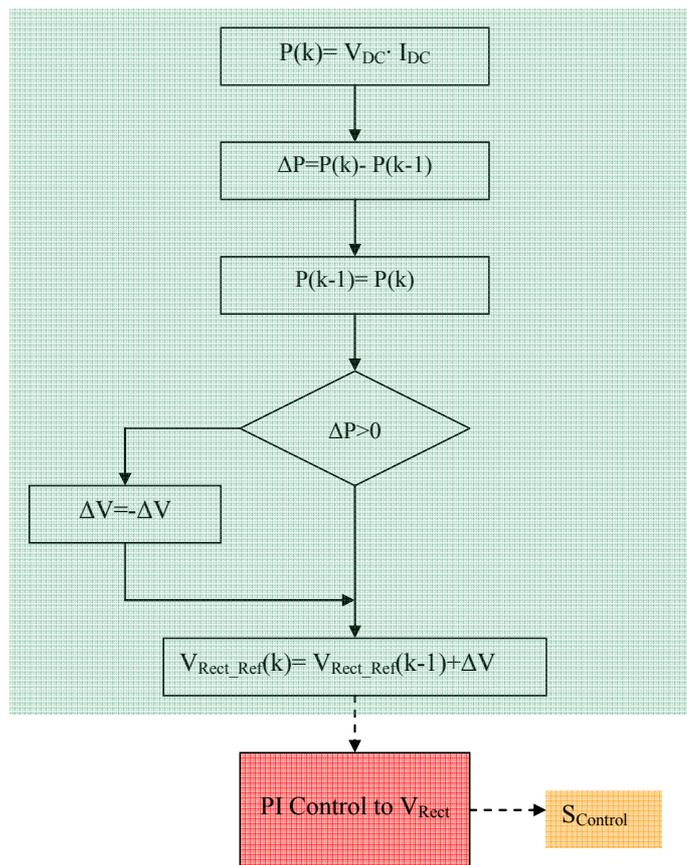
**Figure 51: MPPT to control the DC/DC converter**
