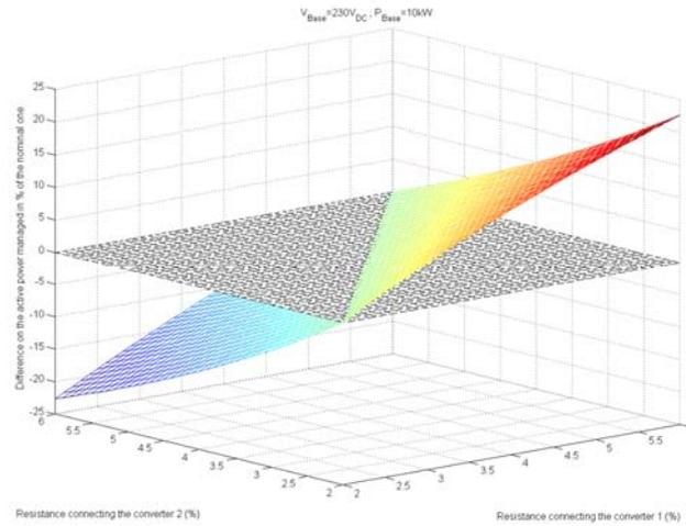
**Figure 10: Difference on the power injected by several inverters connected through unequal resistances**
