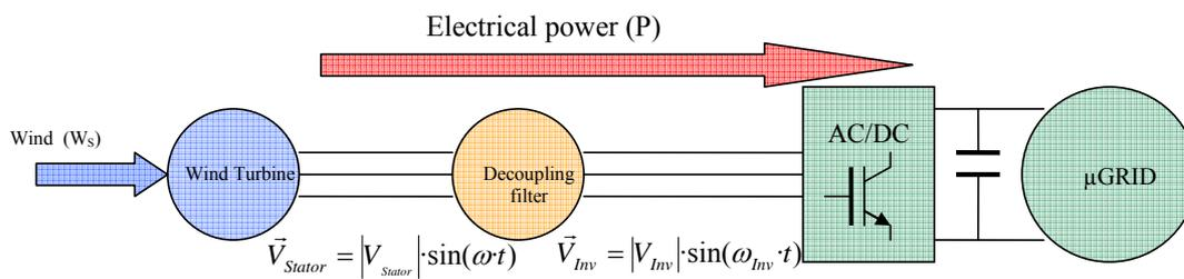
Figure 41: Wind turbine connected to the DC network through an inverter
