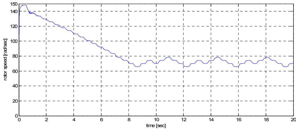
**Figure 44: Rotational speed on the wind turbine rotor**
