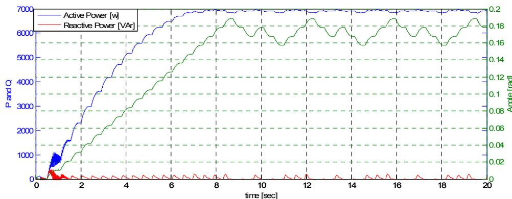
**Figure 43: Active and reactive power and controlled angle of the wind generator**
