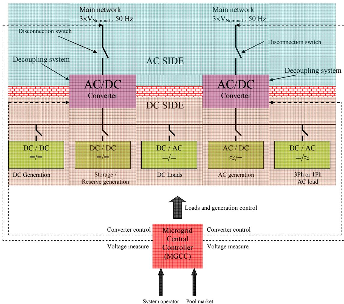
**Figure 7: Topology of the  $\mu$ Grid and connection to the main network**
