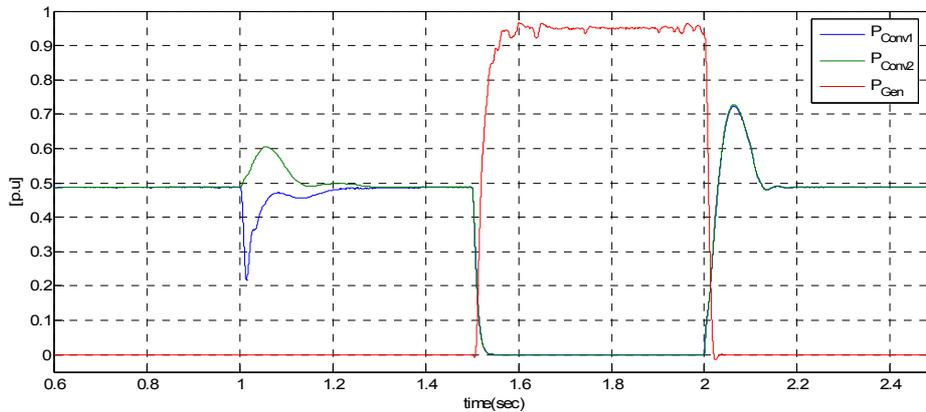
**Figure 31: Power distribution between converters and internal generation**
