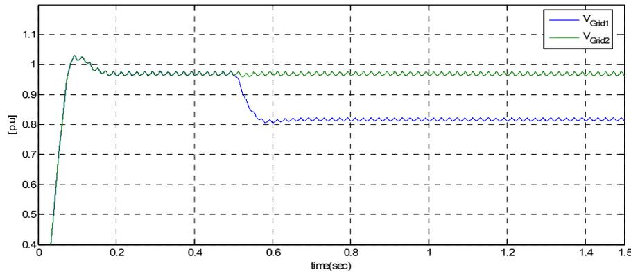
**Figure 19: Voltage drop on the AC side of converter 1**
