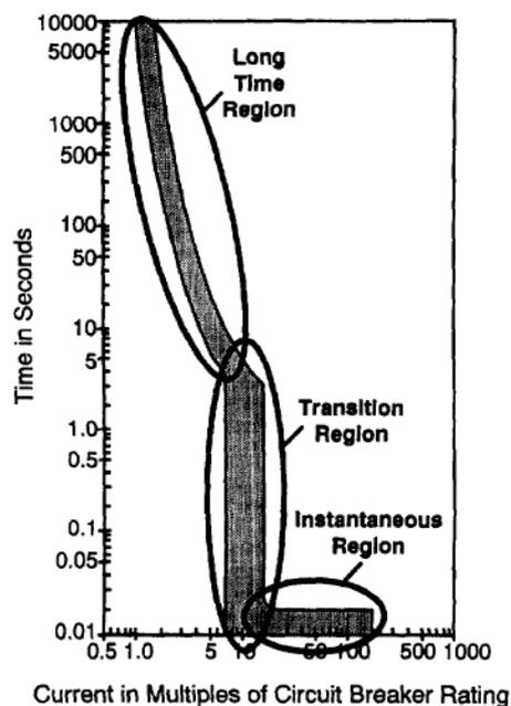
**Figure 35: Typical time-current tripping characteristic for a thermal-magnetic circuit breaker**
