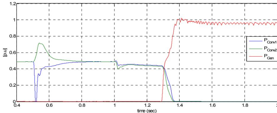
**Figure 26: Distribution between the external and internal active power to guarantee the DC voltage re-establishment**
