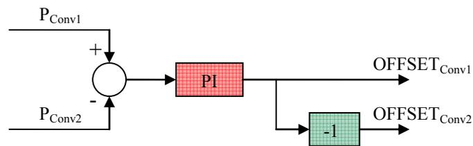
**Figure 16: PI control of the active power mismatched**
