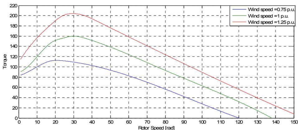
Figure 38: Torque versus rotational speed of a wind turbine for several wind speeds
