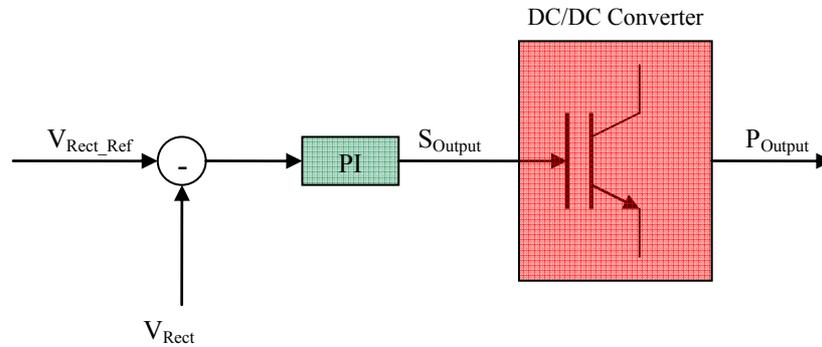
**Figure 52: Adjustment of the MPPT reference voltage with the DC/DC converter**
