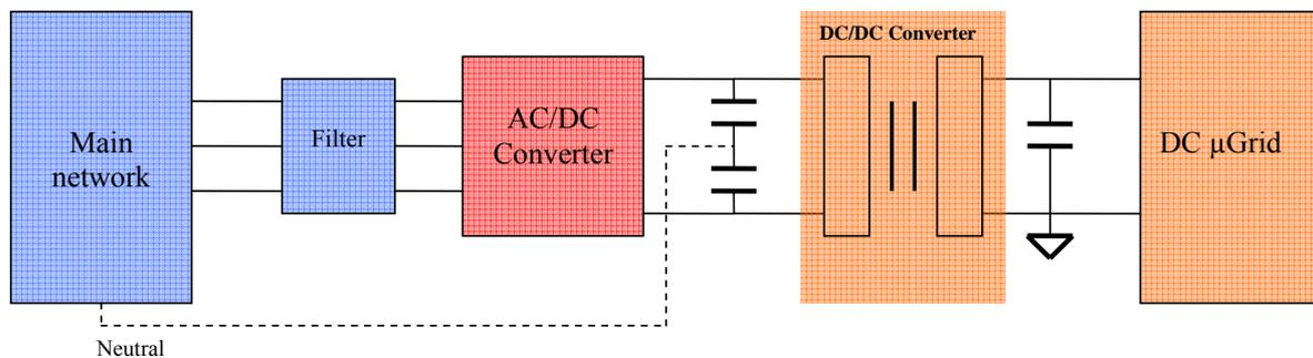
**Figure 34: μGrid isolation through a decoupling transformer on the DC side**
