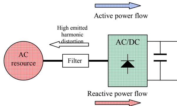
Figure 58: Rectifier based converter
