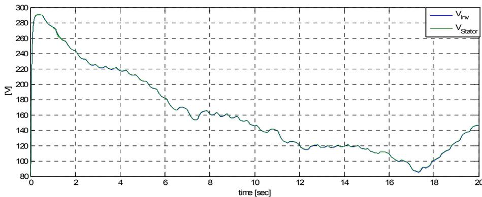
Figure 49: Voltages on the wind generator and inverter
