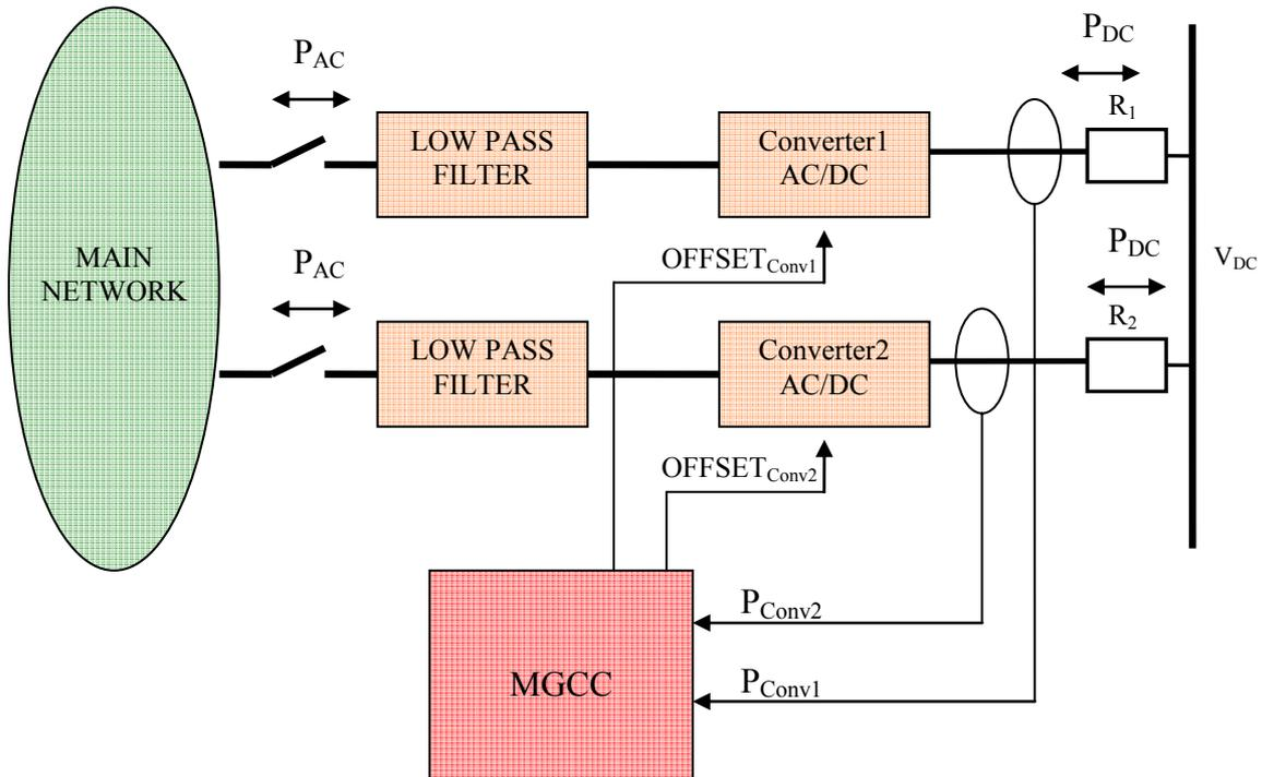
**Figure 15: Equalization of the active power amongst the converters.**
