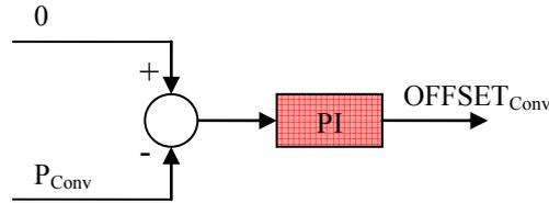
**Figure 24: PI control to null the active power of the main converters**
