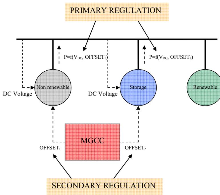
Figure 29: Voltage control in islanded mode
