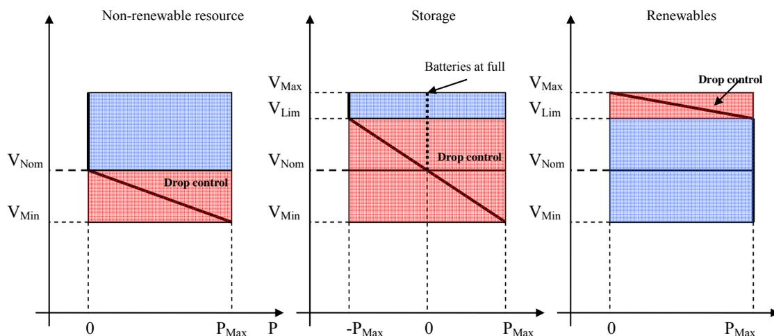
**Figure 28: Voltage control in a DC islanded  $\mu$ Grid**
