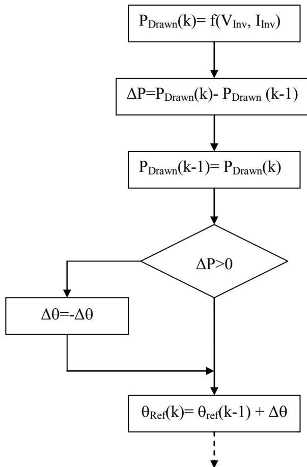
**Figure 40: Simple MPPT technique flow chart**
