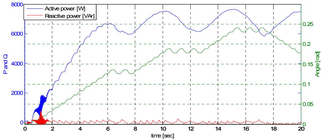
Figure 48: Angle variation to control the active power injection
