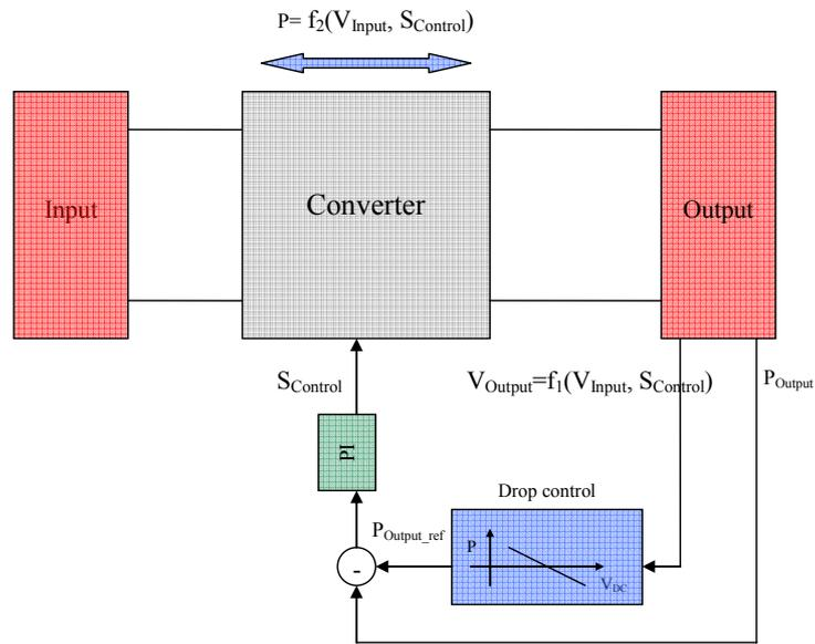
Figure 60: Output power- output voltage control
