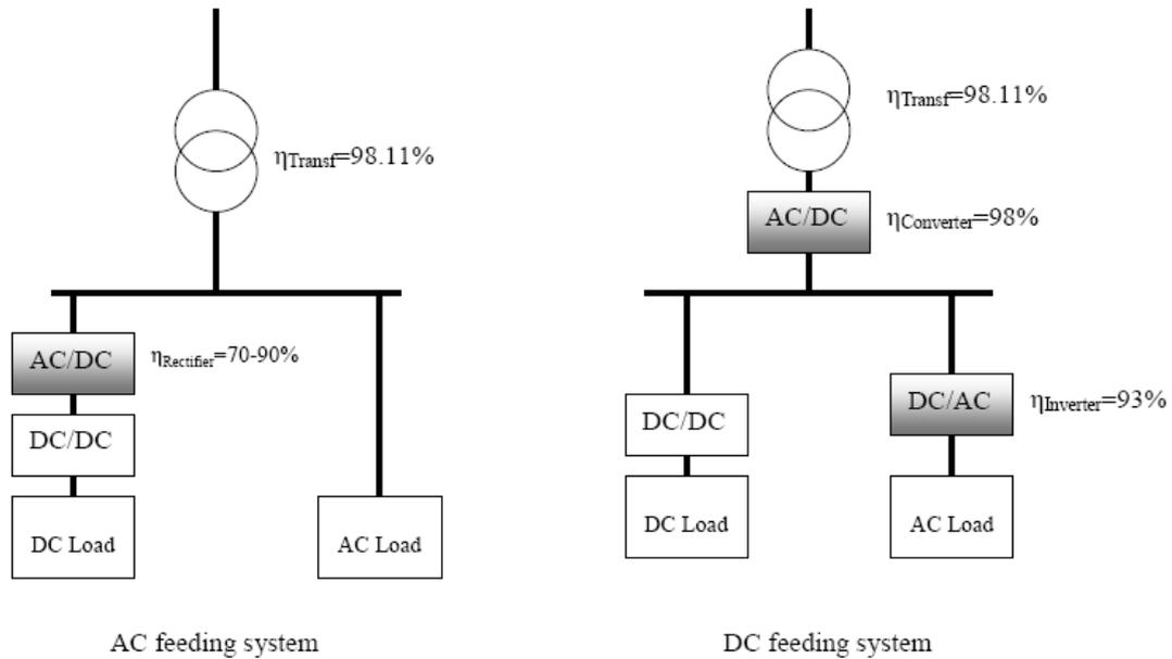
**Figure 5: AC feeding system Vs DC feeding system**
