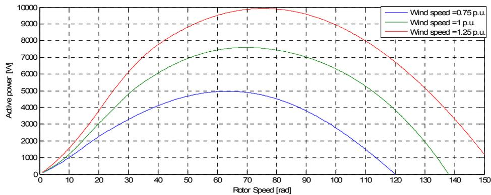
**Figure 39: Active power extracted from the wind as a function of the wind lineal speed and the axis rotational speed**
