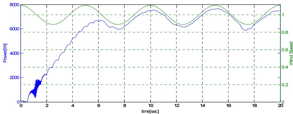
**Figure 47: Wind speed and active power extracted from the wind generator**
