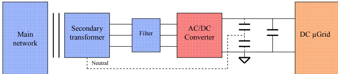
**Figure 33: μGrid isolation through a decoupling transformer on the AC side**
