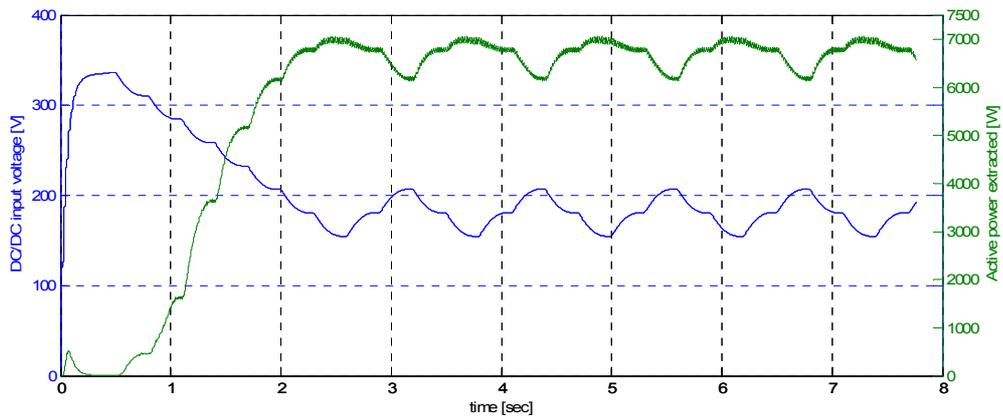
**Figure 53: Reference voltage and controlled active power**
