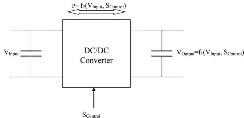
**Figure 59: DC/DC converter**
