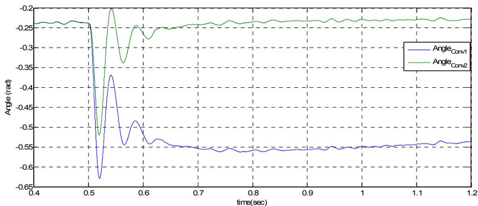
**Figure 20: Angle control of each converter**
