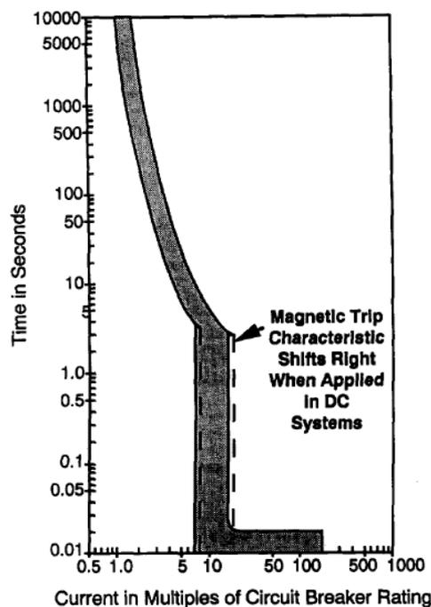
**Figure 36: Characteristic curve for a thermal-magnetic circuit breaker modified for DC applications**
