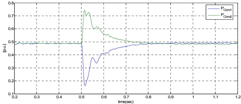
**Figure 21: Active power managed by each converter**
