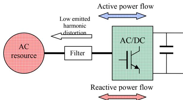
Figure 57: Inverter based AC/DC converter
