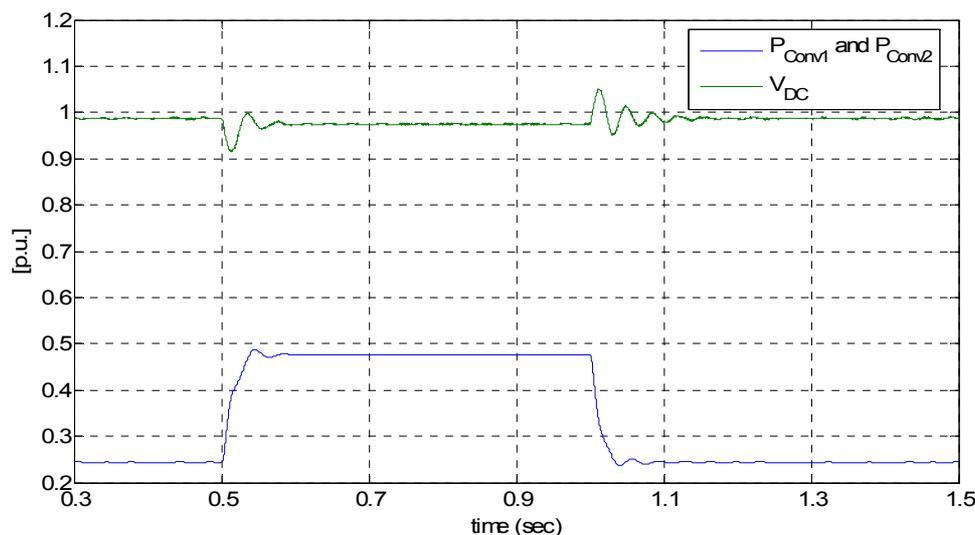
**Figure 13: Equal resistance separating the converters from the  $\mu$ Grid**
