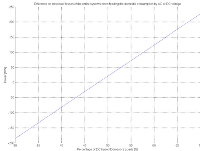
**Figure 6: Difference on the mean losses on the domestic sector when DC or AC supplied**
