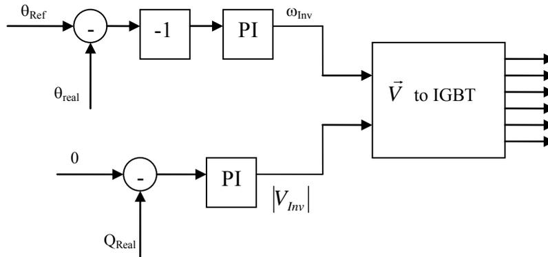
**Figure 42: Power flow control**
