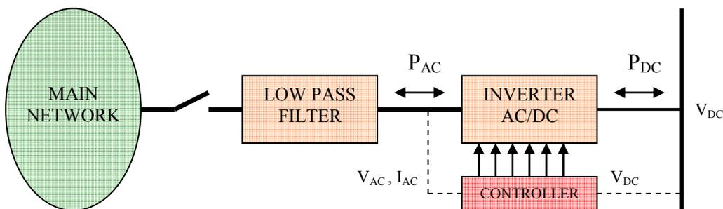
**Figure 11: Inverter based converter connection**
