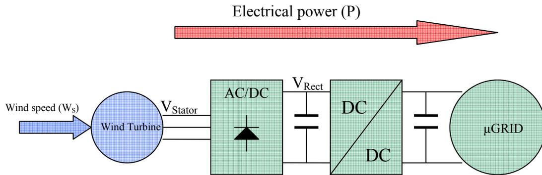
**Figure 50: Wind turbine connected to the DC network through a rectifier plus DC/DC converter**
