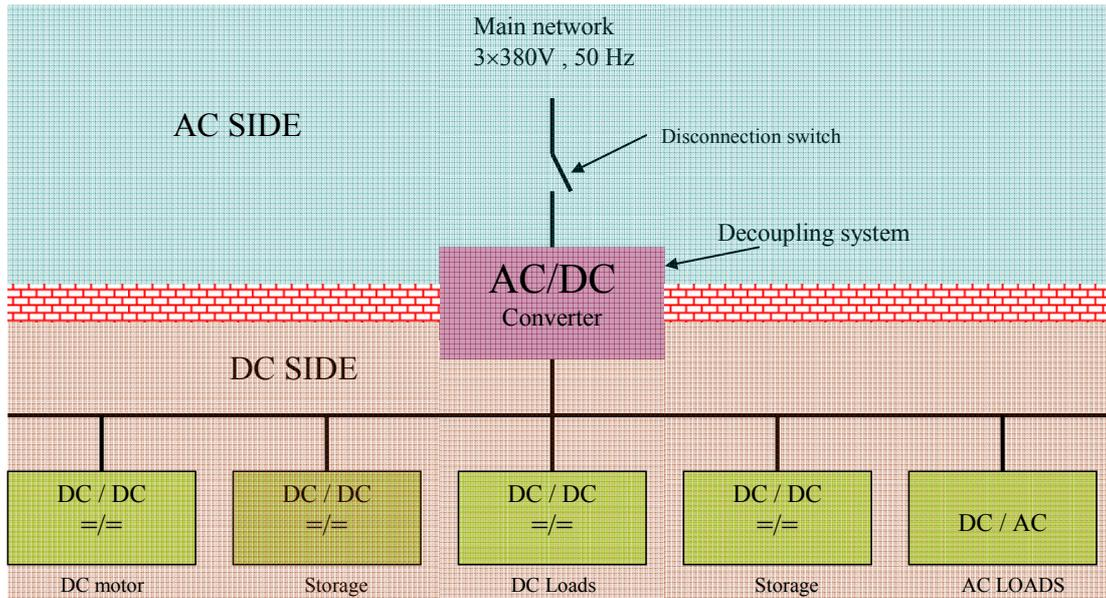
**Figure 37: Load isolation through the AC/DC converter**
