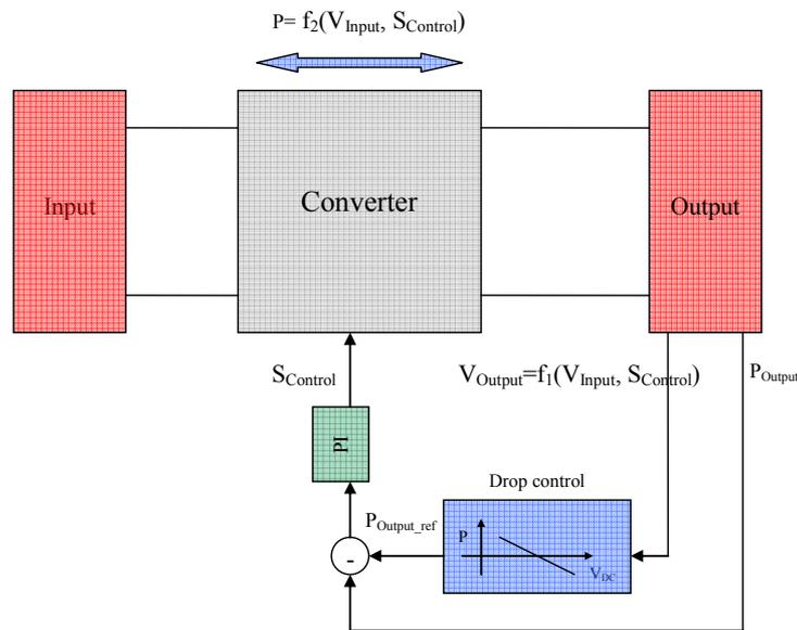
**Figure 25: Primary voltage control of the  $\mu$ Grid in islanded mode**
