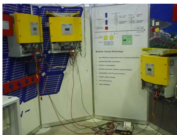
Fig. 29: Two three phase Sunny Island 4500 battery inverter clusters at the DeMoTec with connected Haag measurement devices (see section 4.1.4)
