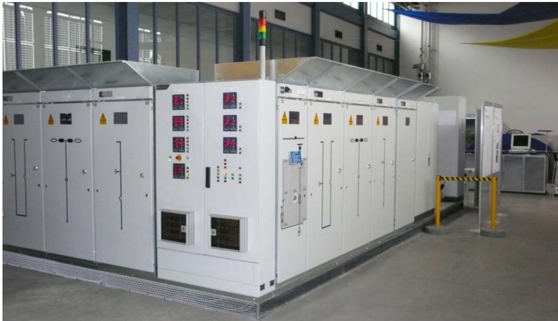
Fig. 26: Line Impedance Simulation Network (LINS) at the DeMoTec
