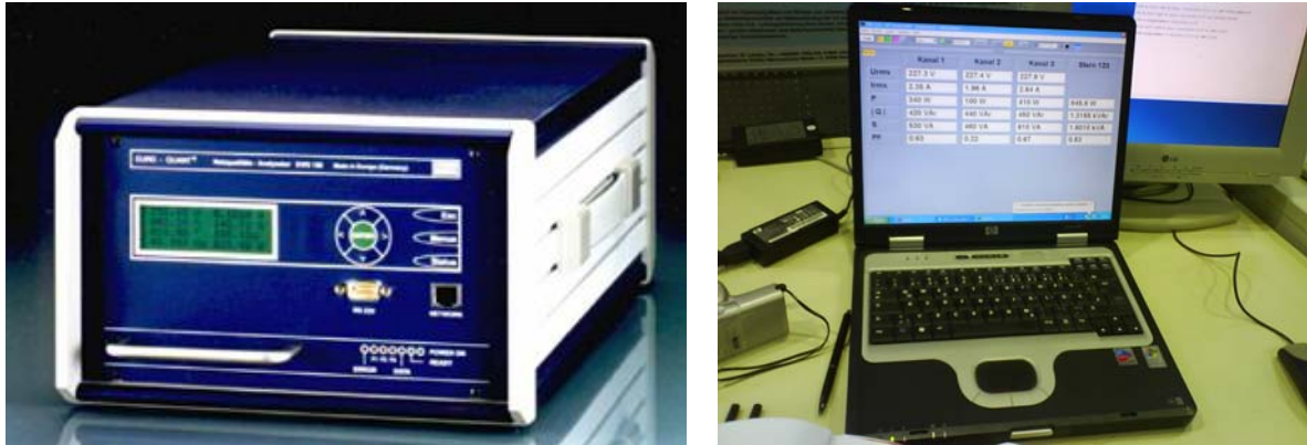
Fig. 33: The “Haag Euro-Quant” device on the left side and the possibility of displaying online measurement values from the devices during the experiment
