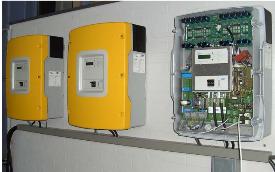
Figure 4-3: Test setup with three Sunny Islands located at DeMoTec lab of Fraunhofer IWES in Kassel.
