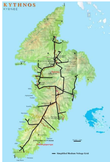
Figure 1: The Medium Voltage distribution line (in black) for the island of Kythnos and the location of RES systems and a microgrid powered by RES in Gaidouromantra (red letters) in the south east side of the island.
