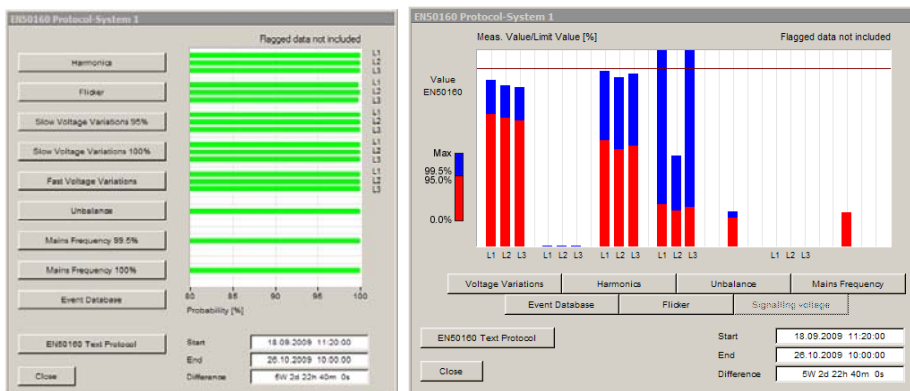
Figure 28 – Voltage compliance analysis with NP EN 50160 standard – 2nd campaign
