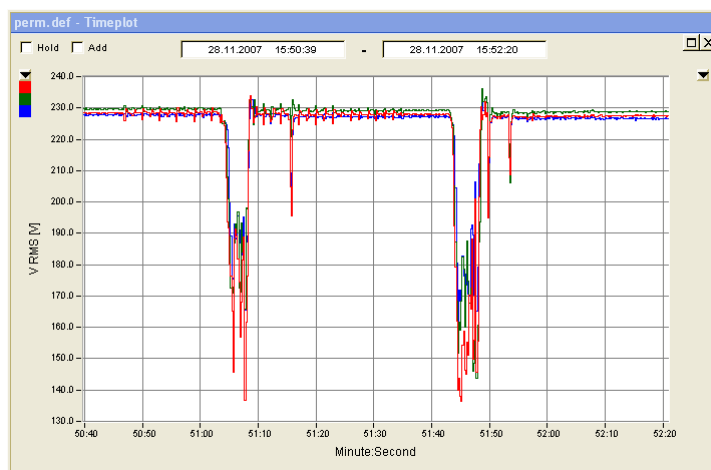
Figure 78 – Voltage RMS values during the connection of the extraction and blowing fans of the ATU 3
