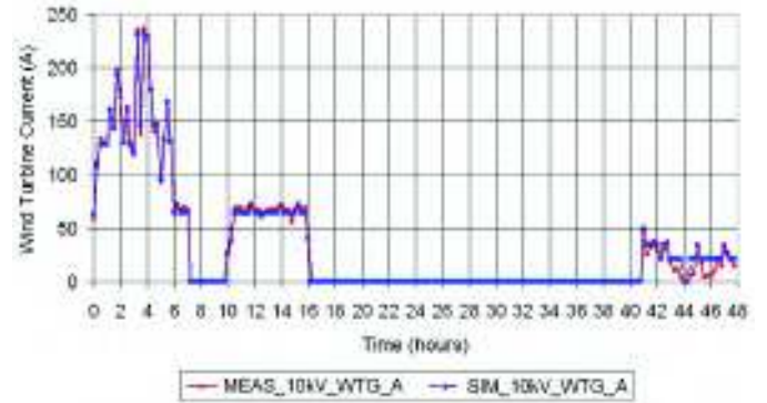
Fig. 6 Measured and simulated wind turbine current (total magnitude) under a 60/10 kV substation during the island operation period
