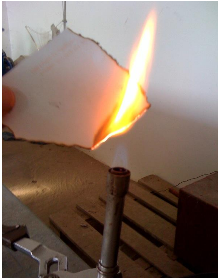
Figure 1 Burning the produced biogas from the Agria farm reactor
