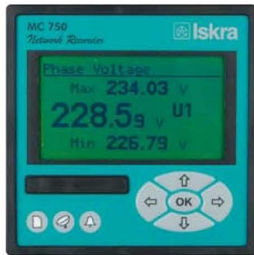
Figure 11 Network recorder – users interface and recorder integrated in a measuring set
