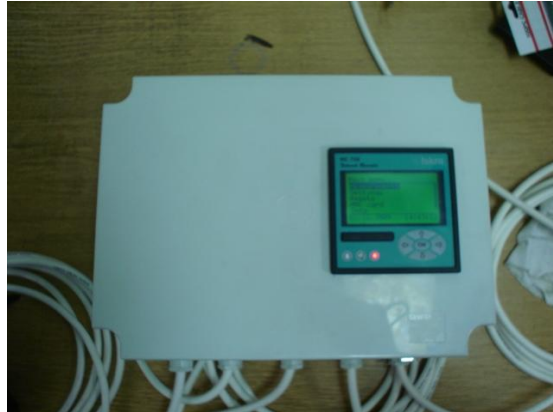
Figure 11 Network recorder – users interface and recorder integrated in a measuring set
