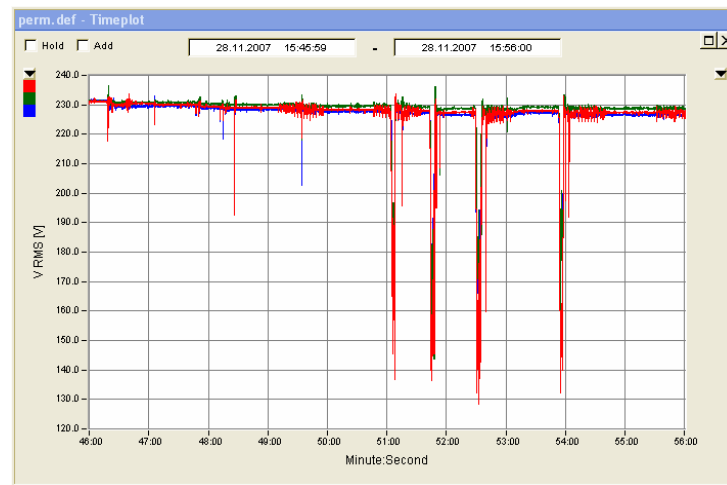
Microturbine output voltage
