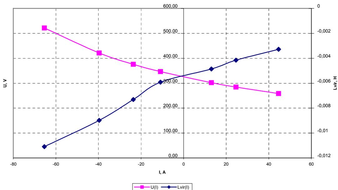
Figure 3-9: U(I) and L<sub>vir</sub>(I) characteristics
