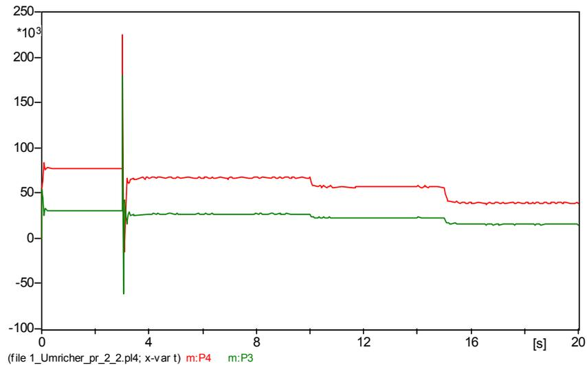
Figure 3-6: Active power contribution (consumption) of the inverters
