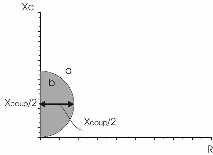
Figure 3-11: Boundary curve for the “self-excitation”: a stability zone; b “self-excitation zone”.
