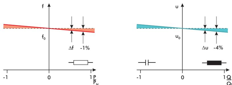
Figure 2-1: Conventional droops in the interconnected grid
