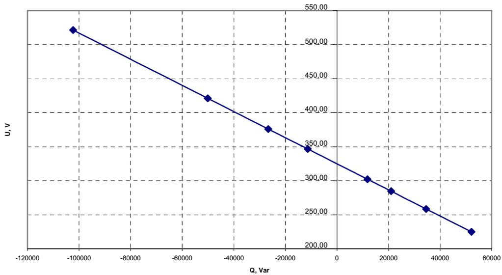
Figure 3-8: Voltage droop:  $k_Q=0,00192$  V/Var and  $R=0,1$  Ohm
