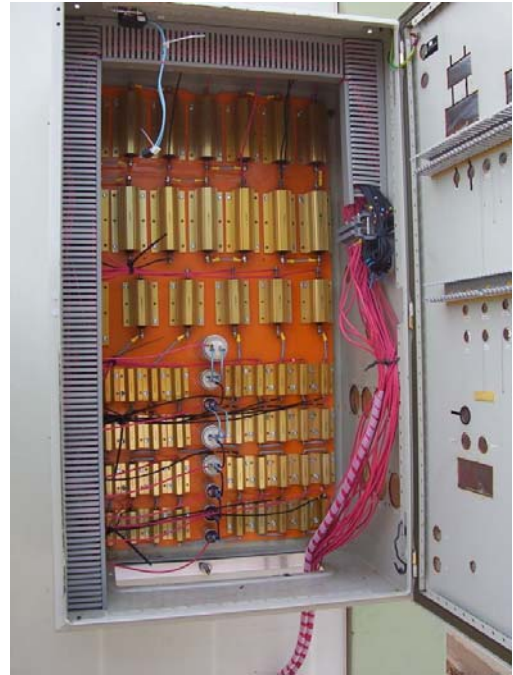
Figure 72: Resistive and capacitive loads
