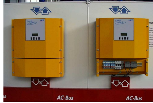
Fig. 4. Two battery inverters SunnyIsland TM by SMA Regelsysteme GmbH, Kassel, Germany operating in parallel (rated power 4.2 kW, clock 16 kHz, coupling inductor 0.8 mH)
