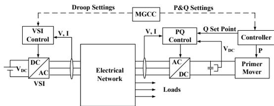
Fig. 6. Control scheme for single master operation
