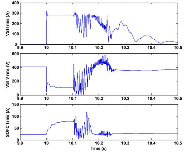
Fig. 12. VSI current and voltage and SOFC current (rms values)
