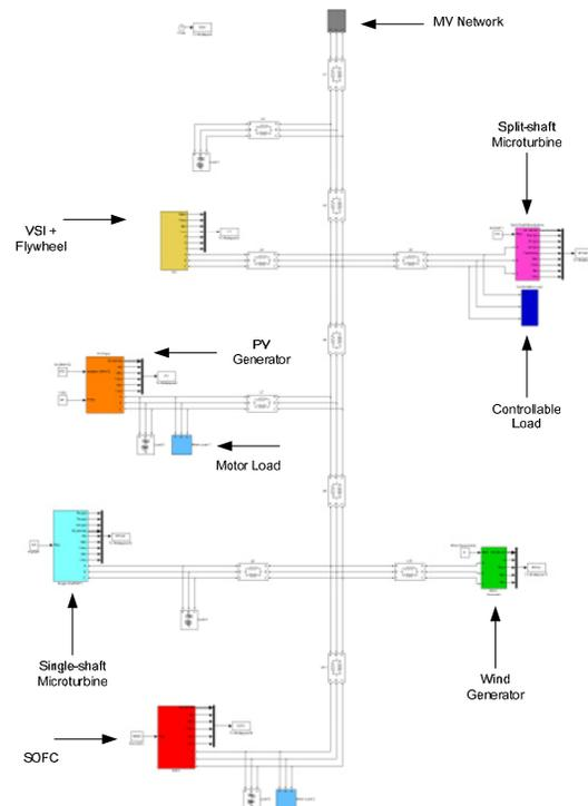
Fig. 9. LV network for the *Matlab® Simulink®* simulation platform
