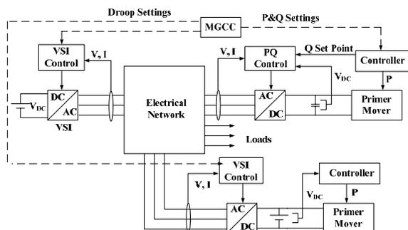
Fig. 7. Control scheme for multi master operation
