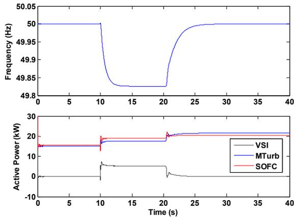
Fig. 13. MG frequency and active power in microsources
