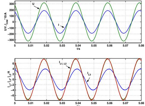
Fig. 5. 3 kW steady state operation; load sharing of three *SunnyIslands*<sup>TM</sup> running in parallel
