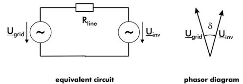
Fig. 6. Resistive coupled voltage sources
