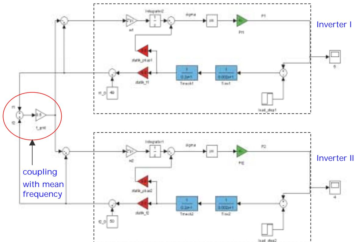
Fig. 5 : Stability assessment based on the system's mean frequency
