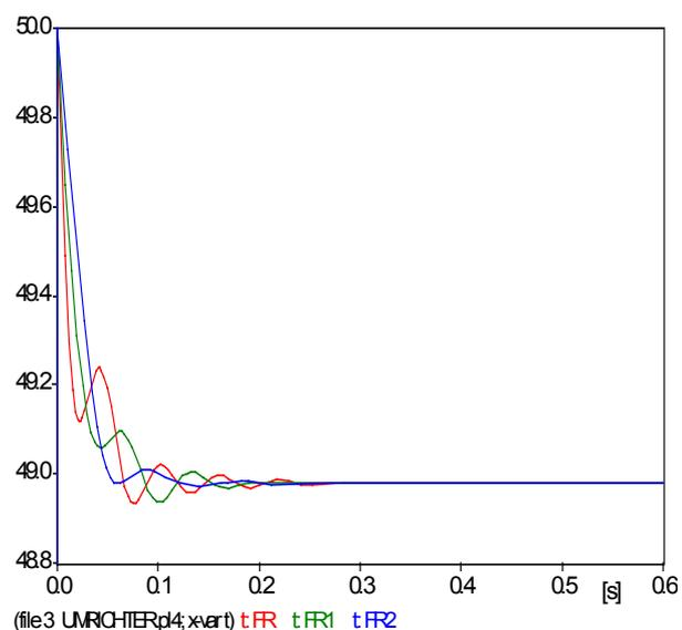
Fig. 4: Frequency change in island system due to load step (100 kW)
