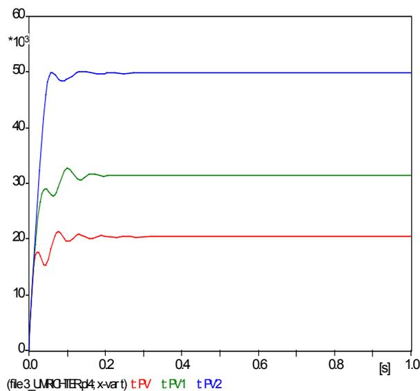
Fig. 3: Load shared between the three inverters (100 kW)
