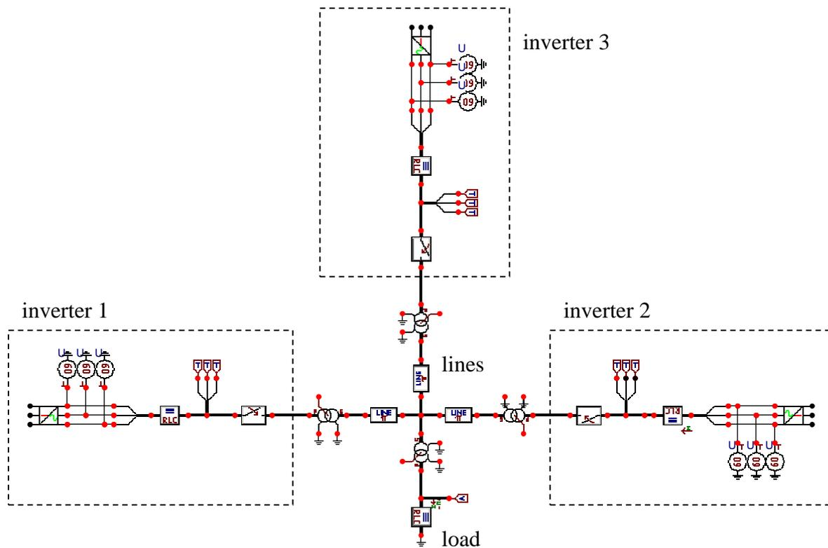
Fig. 2: Simulation of inverter dominated distribution system (ATP-EMTP)
